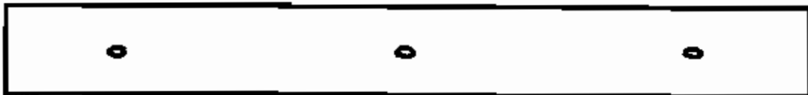
EXAMPLE 3: THREE \frac{1}{8} " (3.2 mm) DISCONTINUITIES
